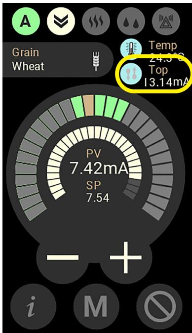
This feature compensates for varying moisture content in the in-take commodity and the feed-out will continuously keep an even moisture content regardless of the in-take moisture content.
