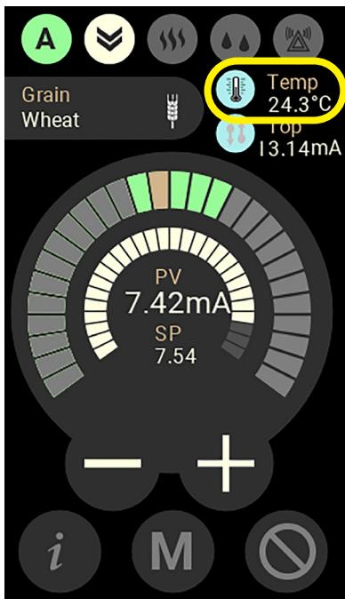
This feature compensates for varying cooling air temperatures and the feed-out will continuously keep an even moisture content regardless of the cooling air temperature.
