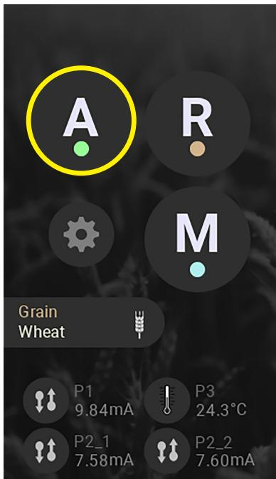
In automatic mode (A) the system internally manages drying times with the help of the PV value (present value) from the main sensor/s and the SP value (set point).
